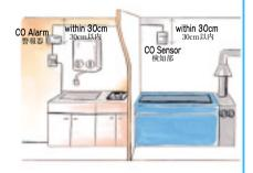
Influences of CO (carbon monoxide) on the Human Body [CO (一酸化炭素)の人体に及ぼす影響] Though LPG (liquefied petroleum gas) itself is not poisonous, its incomplete combustion will produce CO (carbon monoxide). Despite being highly toxic, CO is hardly perceptible due to its physical characteristics—colorless, odorless and nearly the same weight as air. Even the slightest inhalation will cause poisoning leading to death.
