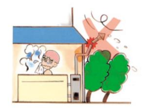
Objects carelessly placed sometimes block exhaust ducts thus causing in complete combustion. Always keep the exhaust duct area in order.
